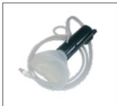
Measuring probe with nose mask
