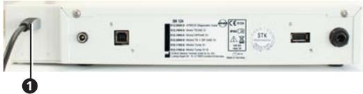
The iHandle is connected to the PC via the USB connection ❶.
