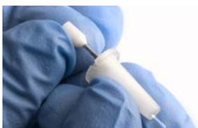
4. Reassemble the probe tip after cleaning.
