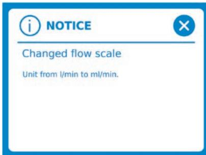
When changing the flow scaling in the long time display to the smallest scaling, the message appears that the scaling unit has changed from l/min to ml/min.
