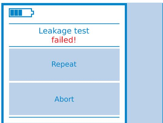
If the leakage test is faulty, the message 'Leakage test failed!' appears. Check the hose connections and whether the secretion canister is correctly clicked into place. By touching the corresponding buttons, you now have the option to:
