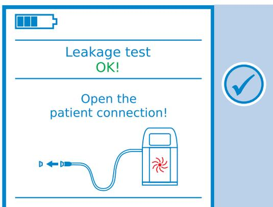
If the leakage test is error-free, the message 'Leakage test OK!' appears. Now you can remove the plug from the hose. By pressing the
