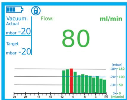
The bar chart appears with a max. flow scaling of 150 ml/min if the average flow value is less than 150 ml/min for at least one hour.
