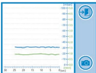
The graphical diagram starts when you call up the menu. In this mode, the real measurements (flow, vacuum) from the last 30 seconds can be shown. Therefore, you can visualise cough tests and other procedures.
