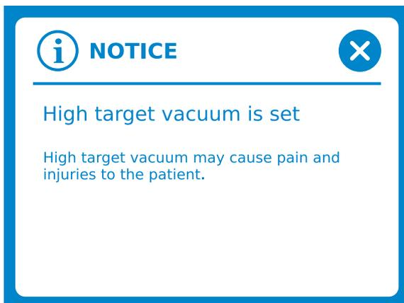
If the target vacuum is adjusted over  $-50$  mbar, the notice 'High target vacuum is set' appears.
