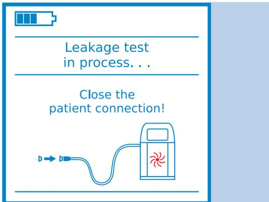
If the leakage test is activated, it will start automatically once the device is switched on. The hose attachment towards the drainage catheter should already be sealed with a sterile plug when starting up the device. Alternatively, the chest tube can be clamped near to the patient. Do not clamp the ATMOS hose system.
