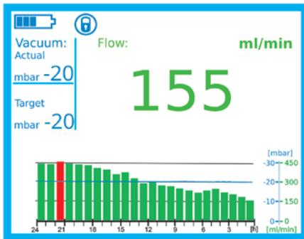
The bar chart appears with a max. flow scaling of 450 ml/min if the average flow value is less than 450 ml/min for at least one hour.
