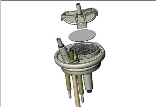
Fig. 32. Lid with bacterial filter plate
